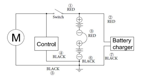
Each column needs two batteries, each battery has one anode "+" and one cathode "-".
