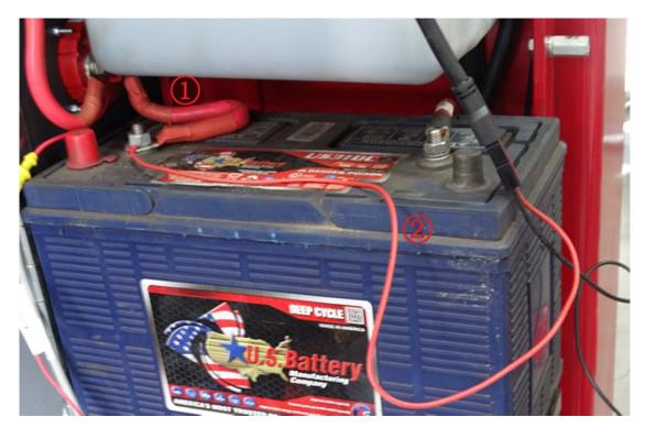
3 Red, connect first battery cathode "-" with second battery anode"+";
